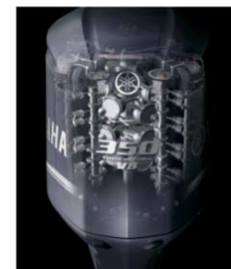
4 - Stroke V8 60 DOHC 32 - valve
