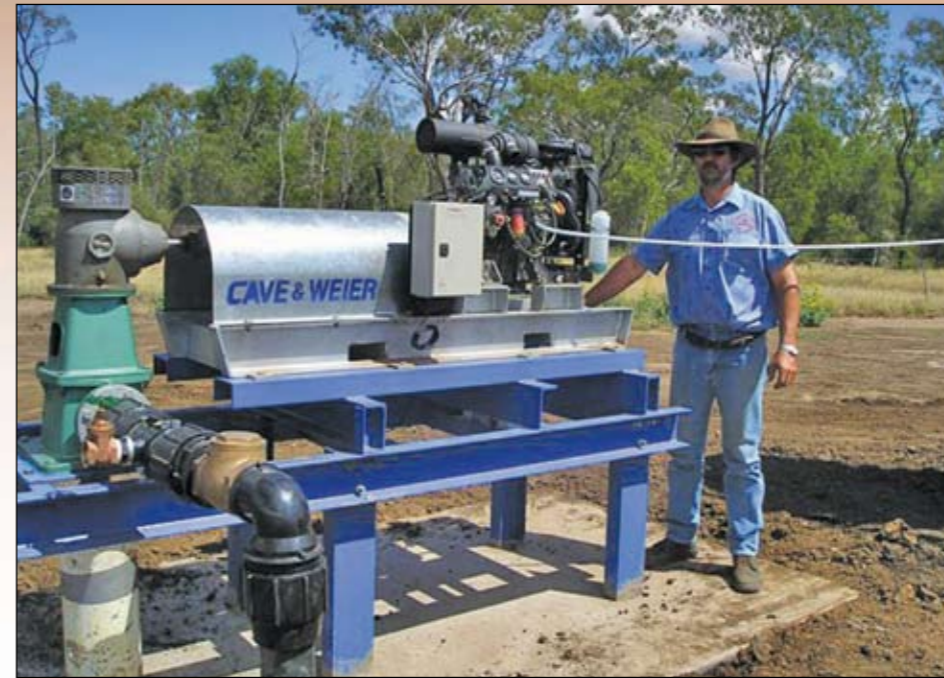
Jeff Weir from McCrackens, Cave and Weir Water Services standing alongside one of the Yanmar powered bore hole pumps
